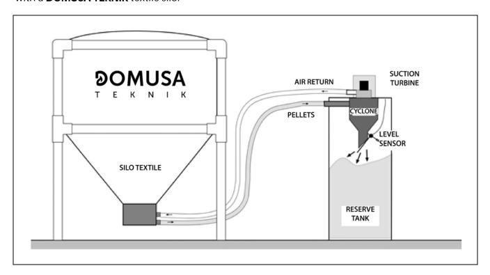
**NOTE:** If the suction system becomes blocked, this could mean there are not enough pellets in the main silo or that the pneumatic hose installation has become blocked or is defective.
