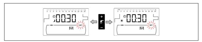
• Press to record the last timer adjustments and it returns to "Configuration" menu.
