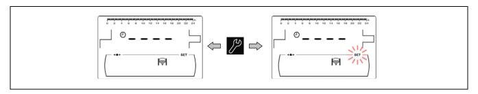
• At the top of the display is shown the time zone, from 0 to 24 hours. Press + / - repeatedly to progress sequentially through the hours every 30 minutes to choose the desired time period.
