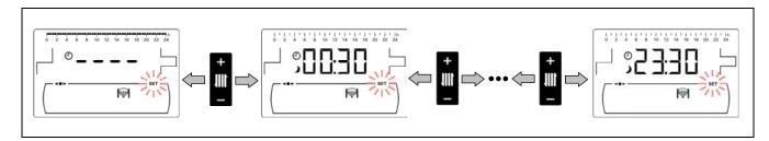
• At each time period pressing + / - the condition of the timer is adjusted. If appears the symbol ")", the Automatic Loading System stays "Off" and if appears the symbol "\* the Automatic Loading System stays "On". The periods adjusted with "\* symbol will be marked in the time zone of the top of the display.
