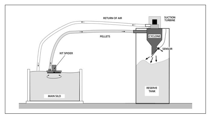
The rotary plate of the **Kit Spider** moves in circular fashion in symmetrical rotation cycles, alternating between clockwise and counter-clockwise movement to prevent the hose from winding onto the kit. These rotation cycles are governed by the **CVS Suction System** electronic control system. The diagram below shows the functioning cycles controlled by the **CVS Suction System**:
