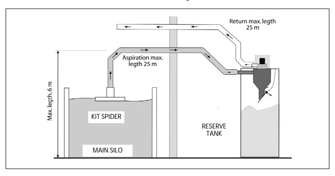
**IMPORTANT:** At each end of the pellet suction and air return hose, the copper cables must be connected to the earth connection terminals provided for this purpose.
