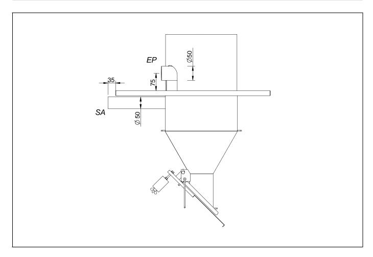
**SA:** Air suction, Ø50. **EP:** Pellet inlet, Ø50.
