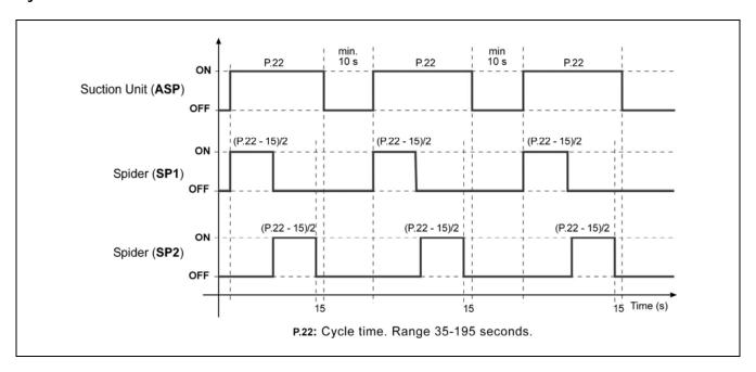
**NOTE:** If the suction system becomes blocked, this could mean there are insufficient pellets in the main silo or that the pneumatic hose installation has become blocked or is defective.
