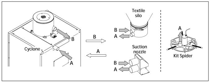
Run a hose from the main storage silo (intake  $\bf A$  of the textile silo or the Spider Kit) to the cyclone (suction pot) on top of the boiler reserve tank and connect it to the intake on the front of the suction pot (intake  $\bf A$ ).
