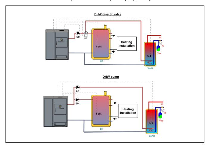
After the hydraulic installation of all the system components, proceed as follows to carry out the correct electrical connection of the BT buffer tank to the **DualTherm** boiler:
