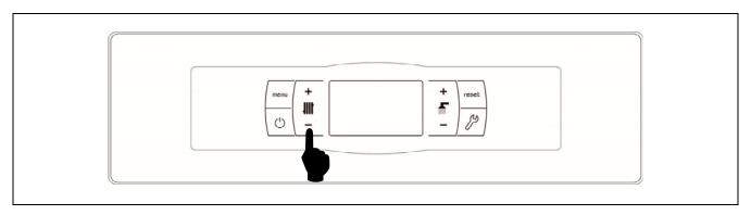
Boiler temperature set point selection is made by the tactile selector shown in the picture. Press "+" and "-" buttons to increase or decrease the set point desired. Few seconds after the desired set point temperature is adjusted the display returns to main position. The range of values for boiler temperature set point is OFF, 75 - 85 °C.
