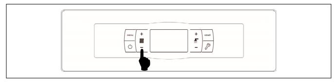
The desired buffer tank temperature is selected using the touch button, as shown in the figure. To select the desired temperature, touch the "+" or "-" symbols to increase or decrease the temperature. When the temperature has been selected, the display will return to standby mode after a few seconds. The permitted range of set point temperature is OFF, 30 - 80 °C.
