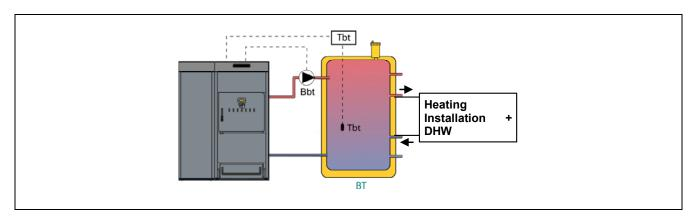
After the hydraulic installation of all the system components, proceed as follows to carry out the correct electrical connection of the BT buffer tank to the **BioClass HM** boiler:
