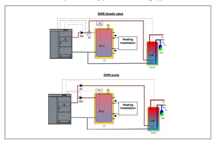
After the hydraulic installation of all the system components, proceed as follows to carry out the correct electrical connection of the BT buffer tank to the **DualTherm** boiler:
