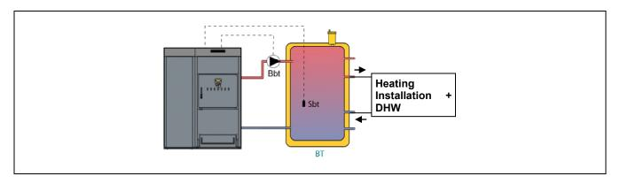
After the hydraulic installation of all the system components, proceed as follows to carry out the correct electrical connection of the BT buffer tank to the **BioClass HM** boiler:
