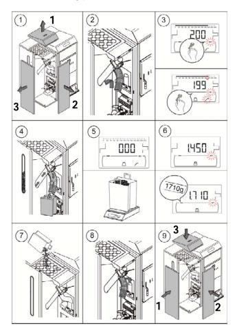
IMPORTANT: Calibrate the feed auger during commissioning of the boiler or whenever the fuel supplier has been changed.
