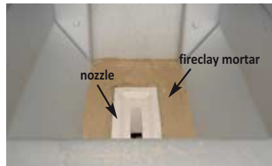
fuel chamber with separate nozzle (from HVS 25 on)
