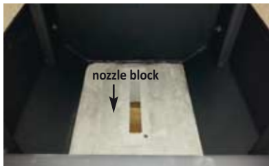
nozzle block with integrated nozzle (only HVS 16)
