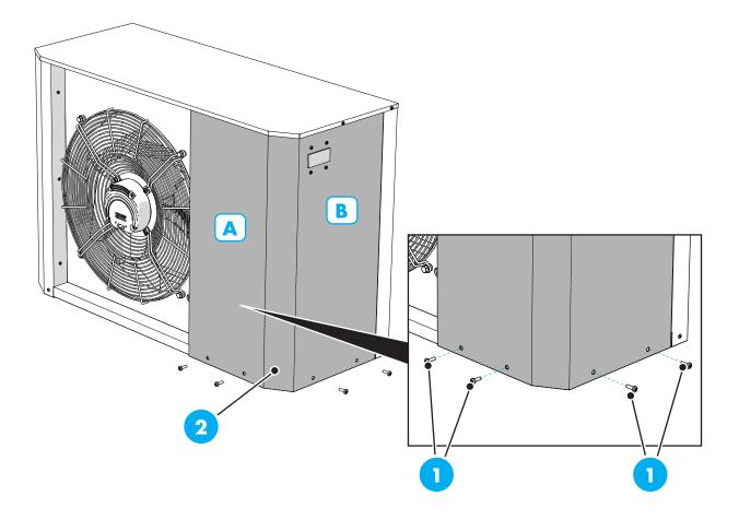
disengage the panel (2) by sliding it outwards;
